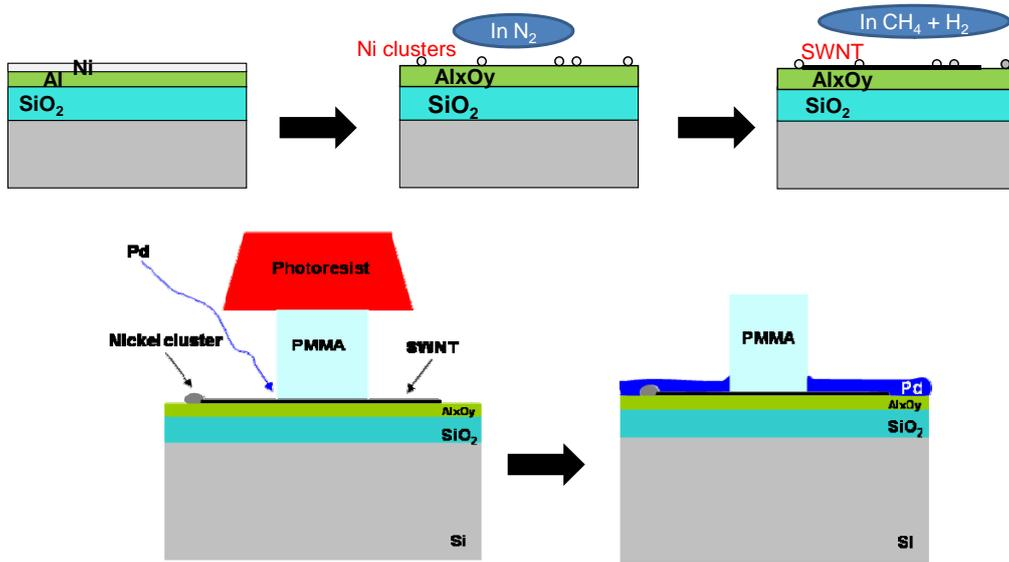
Figure 1. Schematic of the fabrication process for CNTFETs reported in this work.
