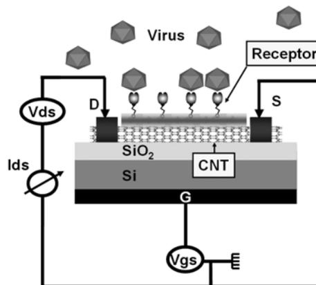
Figure 3. Illustration of proposed CNT sensor for virus detection.
