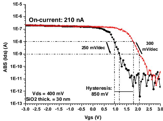
Figure 2. Transfer characteristics of CNTFETs with 30 nm gate oxide thickness.
