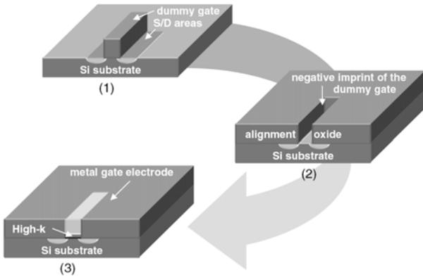
Fig. 1: Main process modules of the replacement gate technology.
