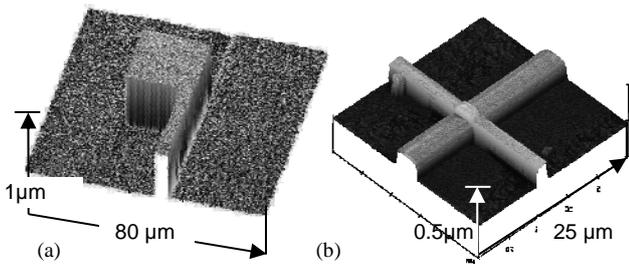
Fig. 2: Atomic force microscopy (AFM) image of a dummy gate structures produced with light optical lithography (a) and electron beam lithography (b).
