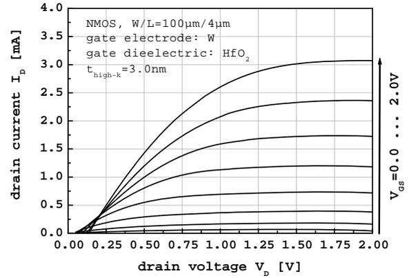
Fig. 4: Output characteristics of damascene metal gate  $\text{HfO}_2$  nMOSFET.
