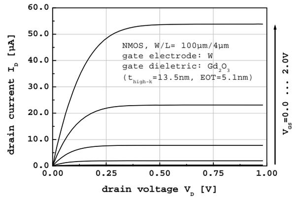
Fig. 5: Output characteristics of damascene metal gate  $\text{Gd}_2\text{O}_3$  nMOSFET.
