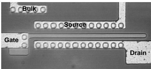
Fig. 3: nMOSFET with high-K  $\text{Gd}_2\text{O}_3$  gate dielectric and tungsten gate electrode realized with the replacement gate process (gate length  $L=4\mu\text{m}$  and gate width  $W=100\mu\text{m}$ ).
