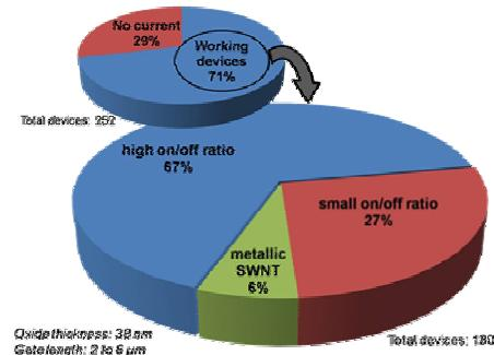
Fig. 2: Nearly 15.000 CNTFET structures have been fabricated. Statistics on hundreds of electrical measurements revealed a total yield of almost 50% (71%  $\times$  67%) for fully functional semiconducting devices, suitable for use as CNTFET memory devices.
