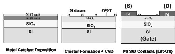
Fig. 1: Process flow of CNTFET memory device fabrication based on CVD with sacrificial catalyst [2].
