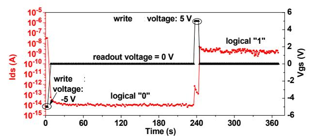
Fig. 4: Cycling of CNTFET memory cell. Black triangles: applied gate voltage versus time. Red dots: measured drain current versus time.
