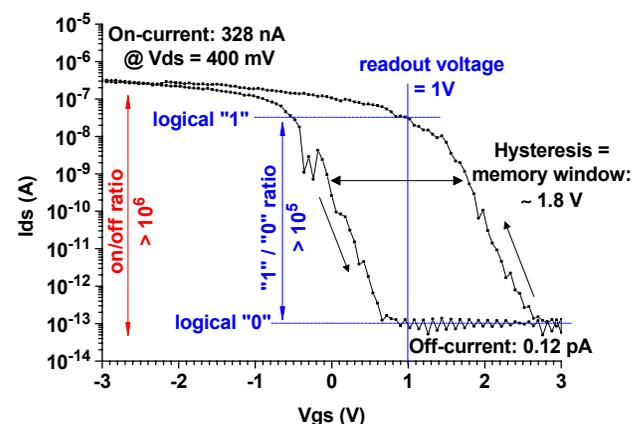
Fig. 3: Example of measured transfer characteristics of fabricated CNTFET device structures with only one s-SWNT as the channel.
